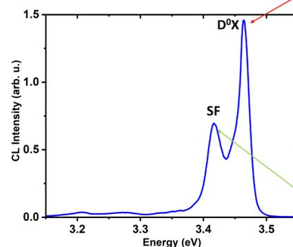
GaN NWs etched in HCl, 15 min. at 90°C.
