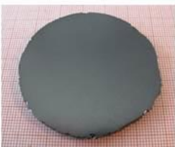
A 2-inch diameter (Cd,Mn)Te single-crystal sample.
