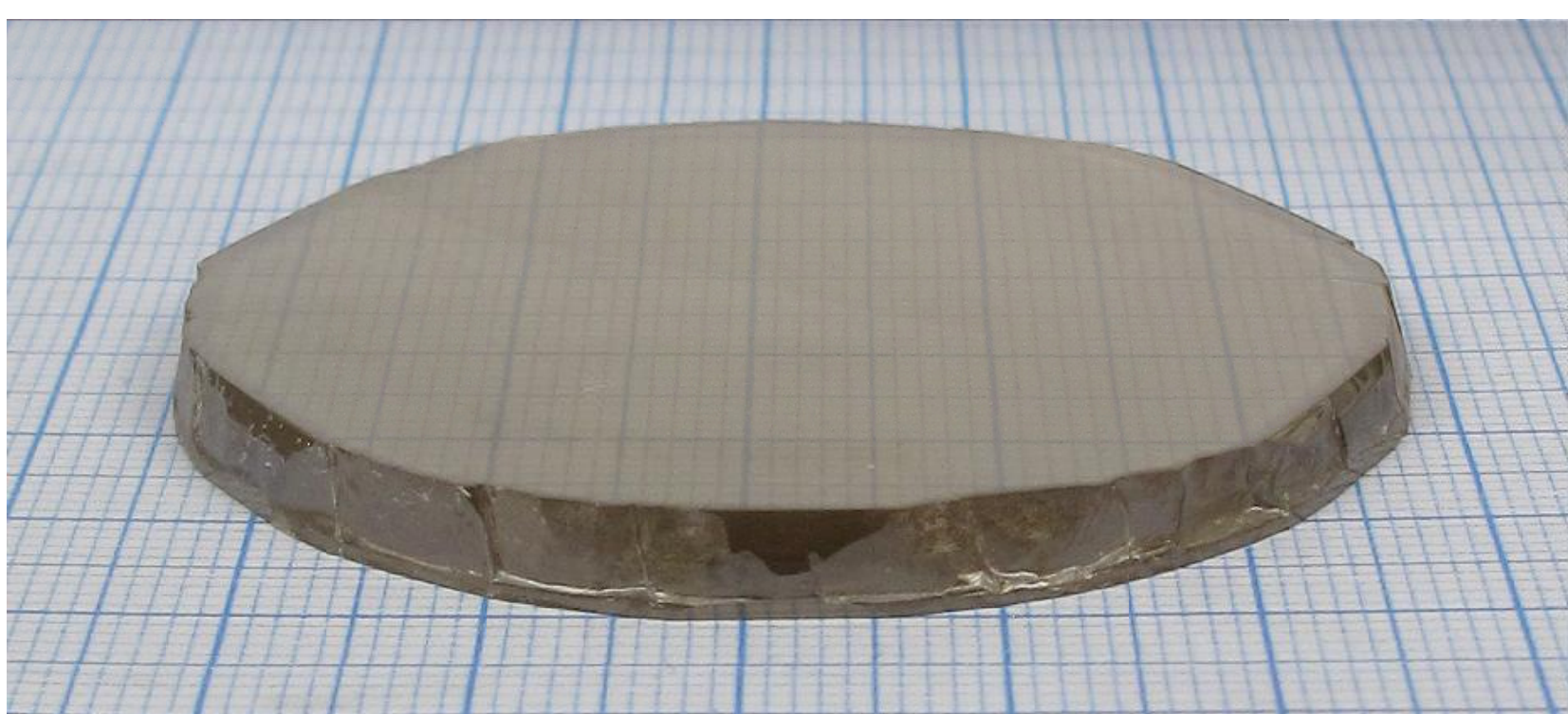
Fig. 2. Ammonothermal-GaN crystal grown in one crystallization run: 6-mm-thick and with a 2.1-inch diameter; grid 1 mm
