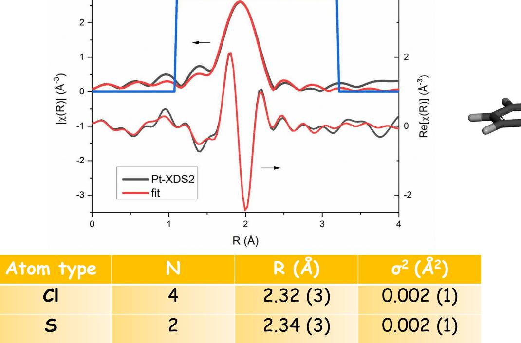
The parameters of EXAFS fitting. N - number of atoms, R - the distance from central atom, σ2 - Debye-Waller factor describing local atomic disorder. The amplitude reduction factor  $S_0^2$  was found to be 0.8 (1) and R-factor of the fit was 0.01.
