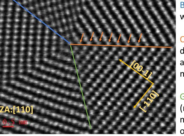
Pb<sub>1-x</sub>Sn<sub>x</sub>Te nanowire with rock - salt
